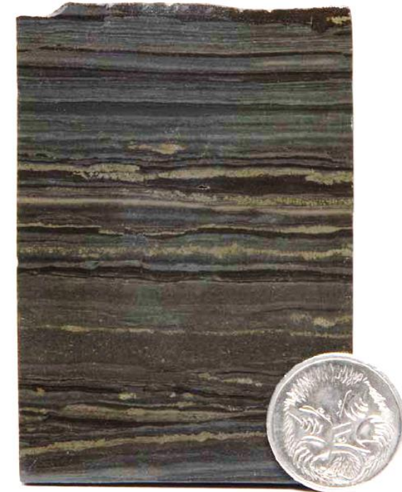
Figure 15.34. Thinly bedded to laminated sphalerite and galena ore typical of the main ore body at McArthur River mine (J Dunster collection).
