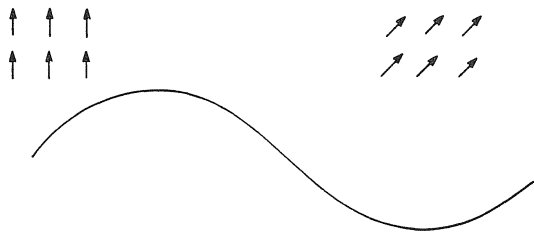
Fig. 8.4. A spin wave inducing a slow spatial variation in the direction of magnetisation in a ferromagnet.
