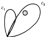
Fig. 3.9. The field-free space in the Bohm–Aharonov effect is not simply connected.
