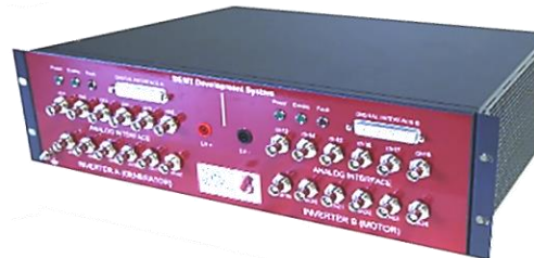
DIS-R3-750-D20 2x10 kW Dual Inverter Stack
