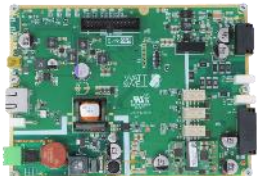
DIS-R3-450-400 100 kW Development Inverter Stack
