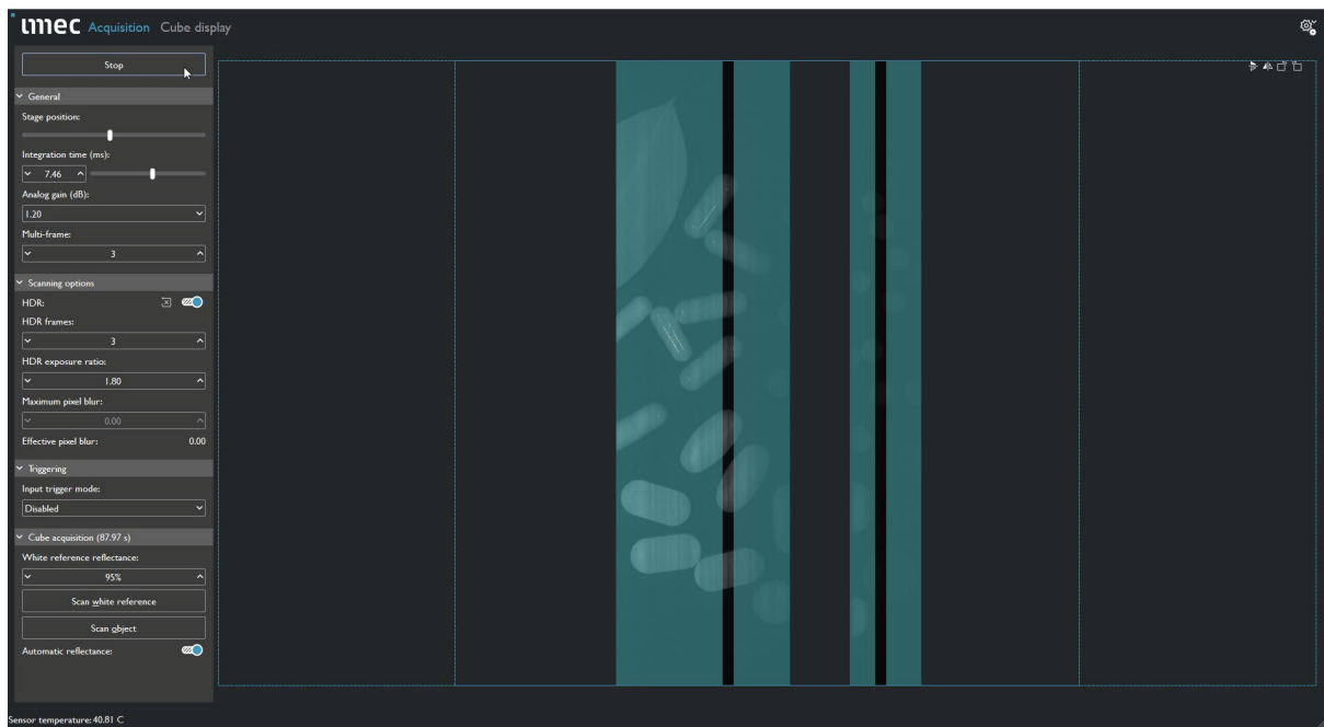
Figure 70: User interface and live view for the acquisition mode after the camera has been connected and configured with specific bands selected. The semi-transparent colored overlay indicates bands that fall outside of the band selection.
