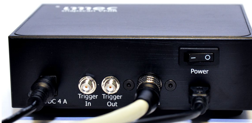
Figure 51 All the connections for the snapscan camera and controller (Step 7.5a)
