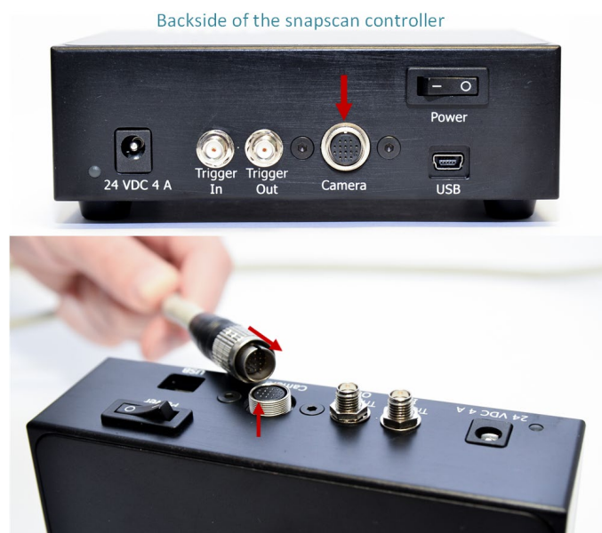
Figure 45 Align the notch on the cable connector to the notch in the controller connector (Step 7.1d)
