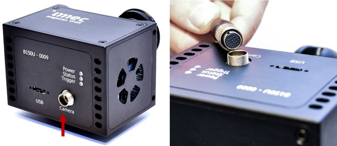
Figure 42 Connecting the 16pin scapscan cable to the camera (Step 7.1a)
