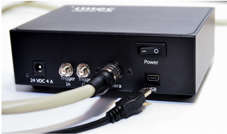
Figure 48 Connecting the snapscan controller to the PC (Step 7.3)
