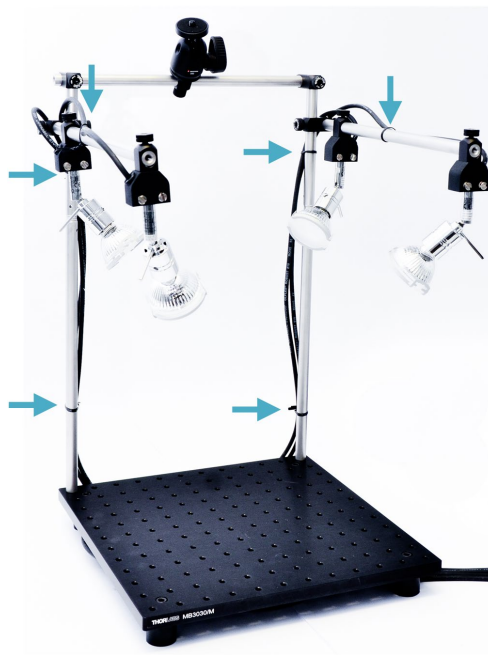
Figure 31 Tying up the loose wires to the mounting posts (Step 4.6)
