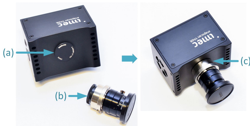
Figure 33 Mounting lens on the snapscan camera (Step 5.1)
