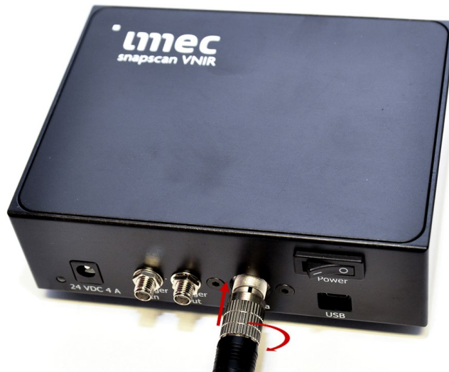
Figure 46 Connecting the snapscan 16 pin cable to the snapscan controller (Step 7.1e)
