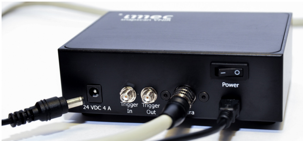
Figure 50 Connecting power adapter to the snapscan controller (Step 7.4b)
