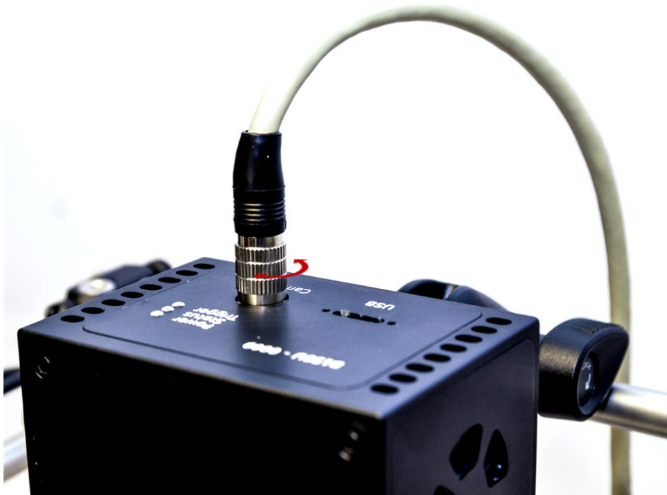
Figure 44 Locking the snapscan controller cable in the camera's connector (Step 7.1c)
