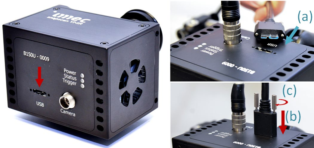
Figure 47 Connecting snapscan camera to the PC (Step 7.2)
