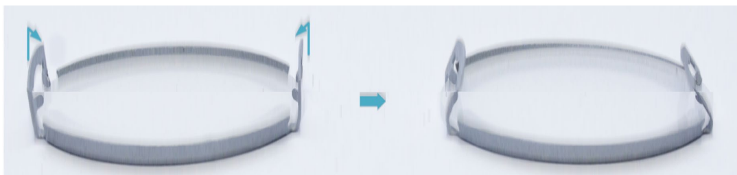
Figure 26 Bending the clips of diffuser for mounting on the lamps (Step 4.3b)
