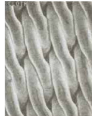
Steel Filter (Ordered Structure)
