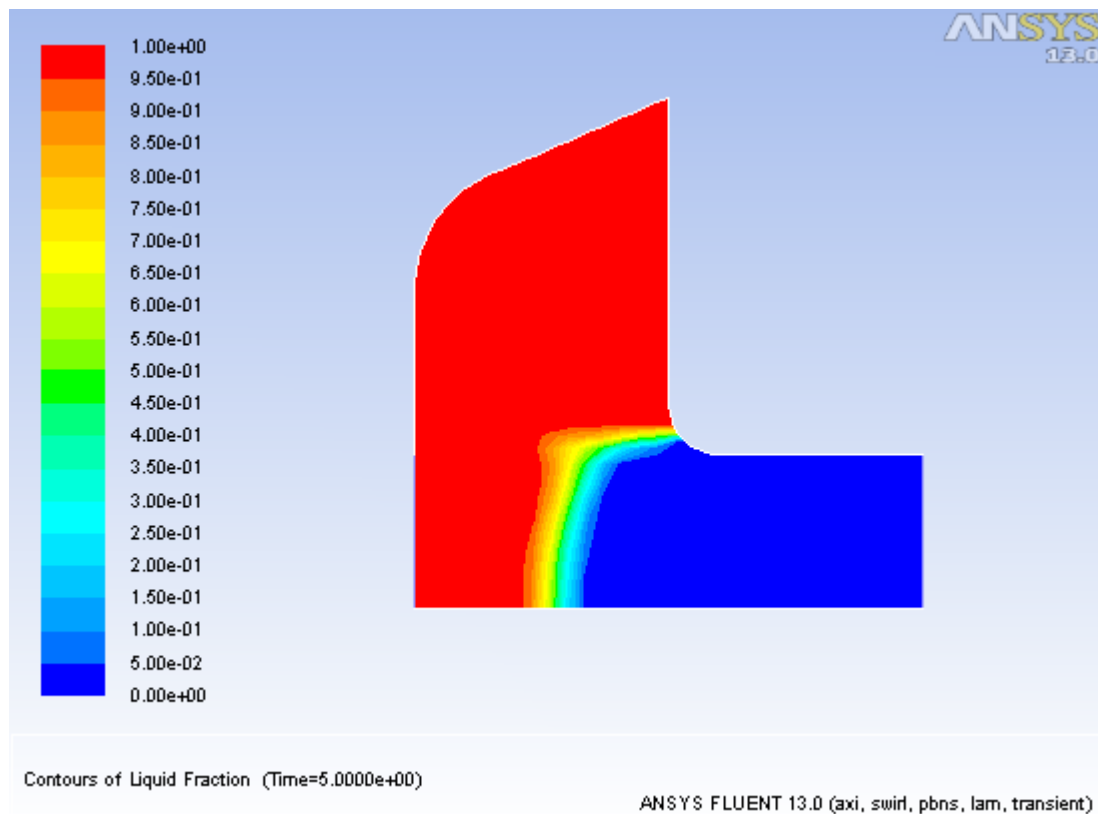
Figure 24.10 Contours of Liquid Fraction at t=5 s
