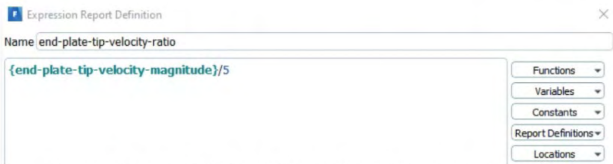
Figure 23.16d) Tip speed ratio definition based on end-plate tip velocity magnitude
