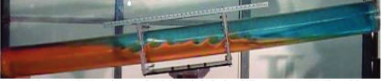
Figure 9.16b) Experiments of Kelvin-Helmholtz instability at t = 5.0 s ( 8^\circ tilt angle), from Matsson and Boisselle 1
