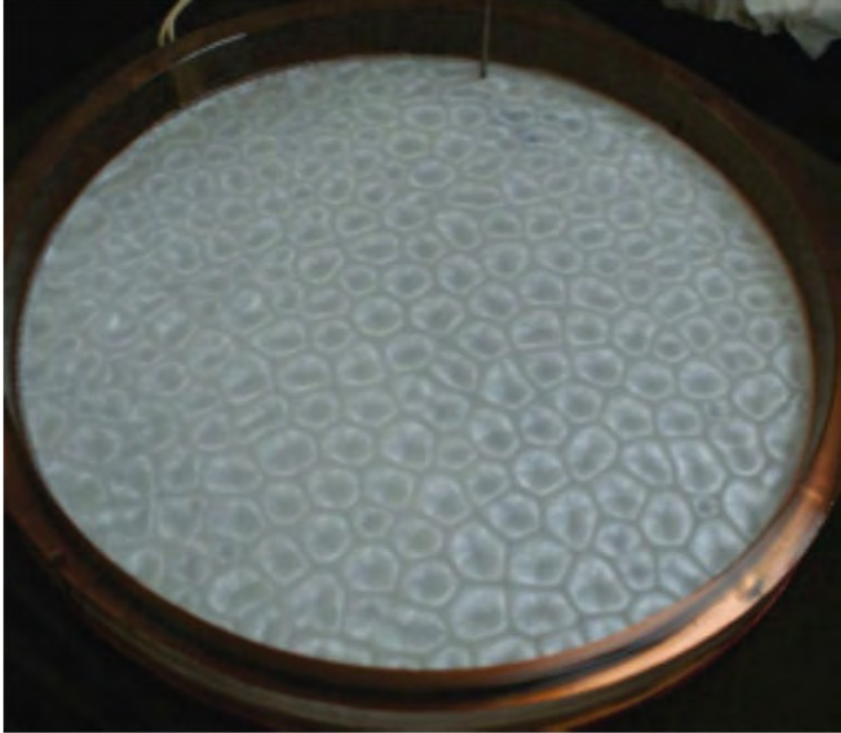
Figure 5.18e) Photo of experimental Rayleigh-Benard convection at Ra = 2120 with a free surface upper boundary condition (copied from Matsson 7 ).
