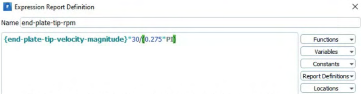
Figure 23.16c) Rotor rpm definition based on end plate tip velocity magnitude
