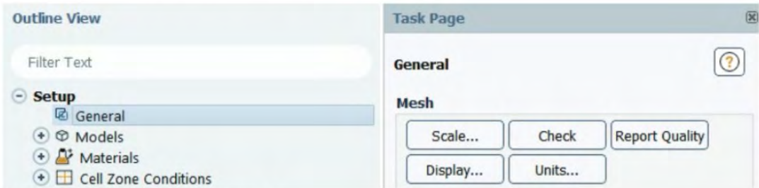
Figure 5.8a) Checking the mesh
