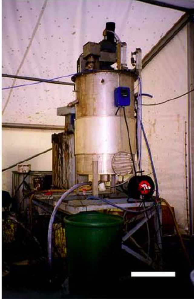
Fig. 4 Photograph of BioMetal Sludge Reactor (BMSR). Marker is 50 cm. Reactor has a volume of 450 L
