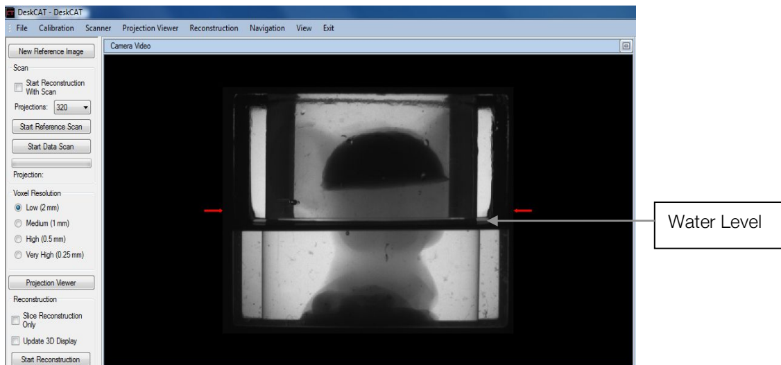
Figure 6: A projection image of a Mouse phantom in a half filled aquarium. Water is a better refractive index match to the phantom than air. Therefore, the effects of refraction are more evident above the water level.
