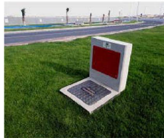
Piezometers installed with dataloggers at different construction sites
