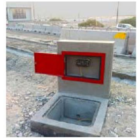
Piezometers installed with dataloggers at different construction sites
